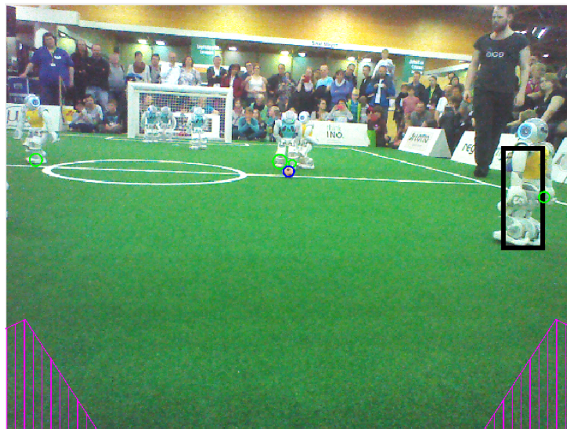
Fig. 2. The robot is able to detect a ball from approximately 4.5 meters distance.
