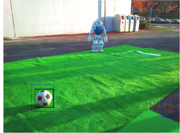
Fig. 2. An example of ball perception under the sunlight exposure in an outdoor environment.
