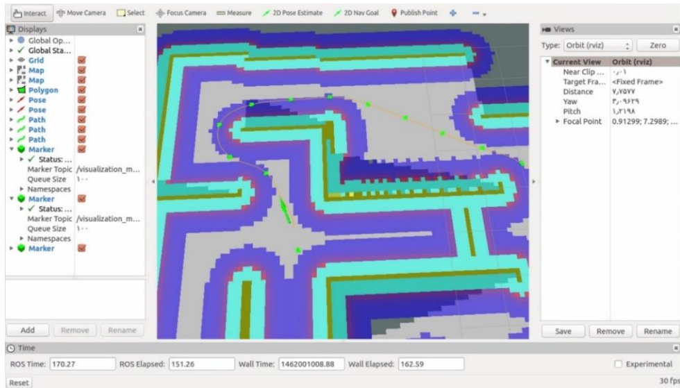
Figure 8. Simulation of our navigation software. The green squares are mid-goals.
