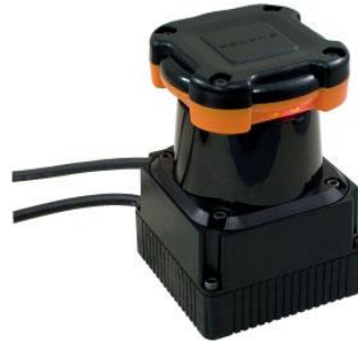
Figure 5. Hokuyo UTM-30LX laser scanner
