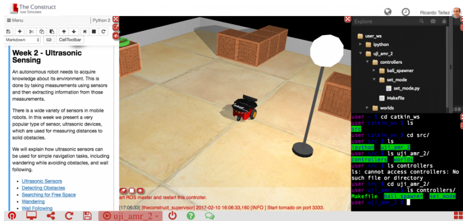
Fig. 1. User interface: from left to right, notebook, simulator view, file editor (top) and shell (bottom).
