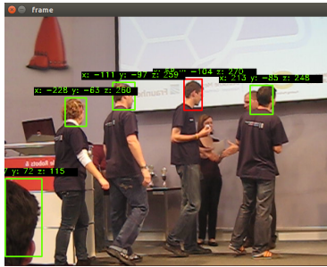
Fig. 5: User interface of the head tracker. Detection bounding boxes in green, tracking target in red. Displayed over each is the head position in world space coordinates in relation to the camera sensor.
