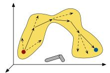
Fig. 5. The planner gives an approximation of actions, (yellow region) that must be refined by trial and error learning into precise motor actions (arrows).
