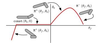
**Fig. 2.** Qualitative Models for the Negotiator Robot, describing the relationship between the angle of the flippers,  $\theta_f$ , and base,  $\theta_b$ , through four operating regions.
