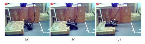
Fig. 1. The Negotiator robot reversing up a high step
